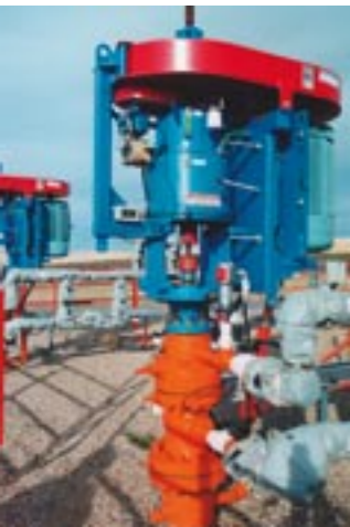
Crude oil production with PC pumping system
